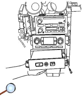
3. Install the communication interface module screws.
